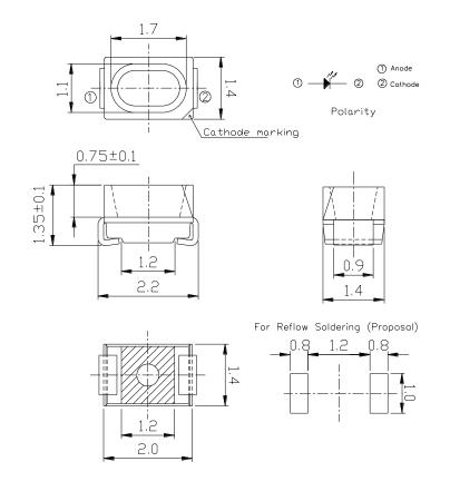
**Notes:** 1.All dimensions are in millimeters 2.Tolerances unless dimensions ±0.1mm
