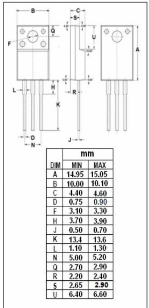
**isc N-Channel MOSFET Transistor**
