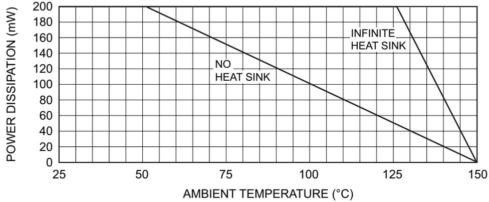
Typical Degradation Curve
