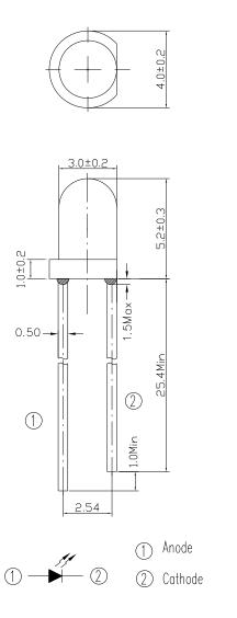
Note: Tolerances unless dimensions ±0.25mm
