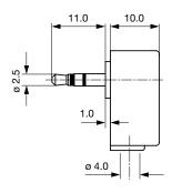
Cable diameter max. 4.0 mm
