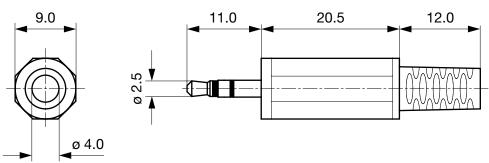
Cable diameter max. 4.0 mm
