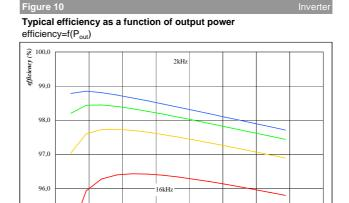
$\begin{array}{lll} \mbox{\bf At} & & & & \\ T_j = & 125 & & ^{\circ}\mbox{\bf C} \\ \mbox{\bf DC link} = & 600 & & \mbox{\bf V} \\ \mbox{\bf Mi} = & 1 & & \\ \mbox{cosfi} = & 0,80 & & & \\ \end{array}$
