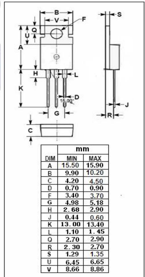
**isc N-Channel MOSFET Transistor**
