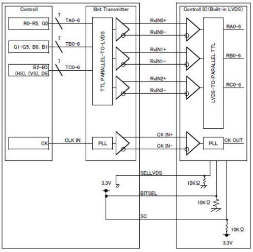
$\mbox{\ensuremath{\$}SELLVDS}$  signal line has 10 k  $\Omega$   $\mbox{\ensuremath{$\mu$}}$  pulldown resister.
