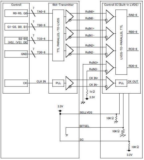
When using "6-bit Transmitter", please connect the unused channel of the control IC receiver as described in the diagram below.
