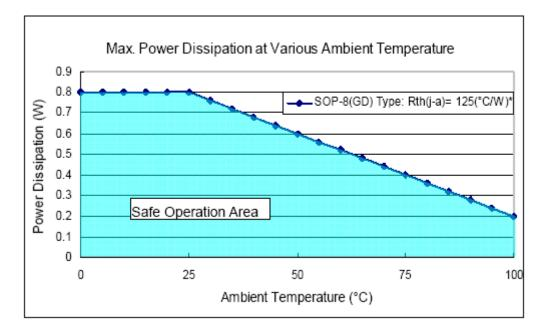
The maximum power dissipation,  $P_D(max) = (T_{j,max} - T_a) / R_{th(j-a)}$ , decreases as the ambient temperature increases.
