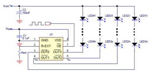
\*VLED = VDS + VFLED x n; VFLED: Forward voltage of LED; n: LED count
