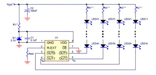
(a) IK2804 application circuit, where  $V_{\text{LED}}$  and  $V_{\text{DD}}$  share a single voltage source.
