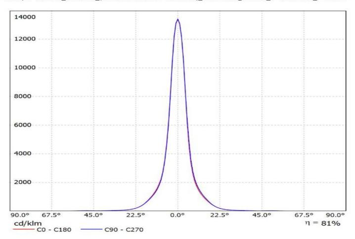
Luminaire: Ledil CP15212\_CARMEN-S-B\_(CXA1507) Lamps: 1 x Cree\_CXA1507-30F-F4-N0H-00000\_BJB\_47.319.6100\_231.805Im@50mA\_P=1.7044W\_I=0.05A
