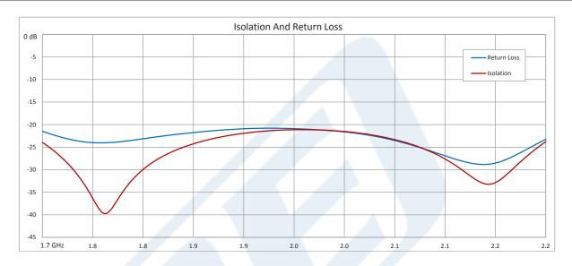
High Power Isolator With 20 dB Isolation From 1.7 GHz to 2.2 GHz, 50 Watts And N Female from Pasternack Enterprises has same day shipment for domestic and International orders. Our RF, microwave and millimeter wave products maintain a 99% availability and are part of the broadest selection in the industry.
