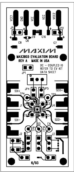
Figure 2. MAX3805 Component Placement Guide
