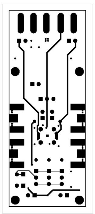
Figure 6. MAX3805 PC Board Layout – Solder Side
