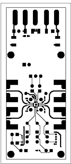
Figure 3. MAX3805 PC Board Layout – Component Side
