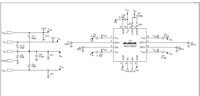
Figure 1. MAX3805 EV kit Schematic
