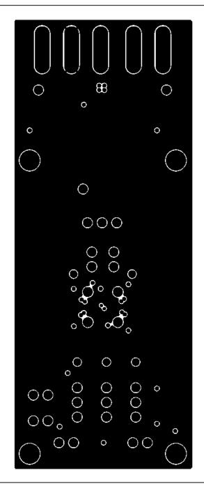
Figure 4. MAX3805 PC Board Layout – Ground Plane
