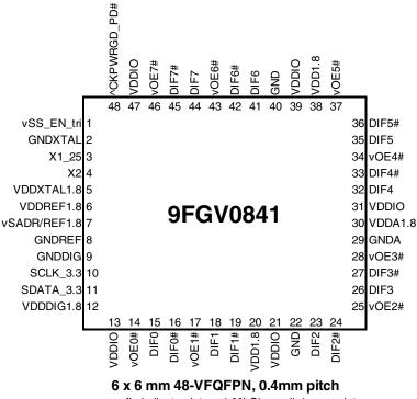
vv prefix indicates internal 60kOhm pull-down resistor
