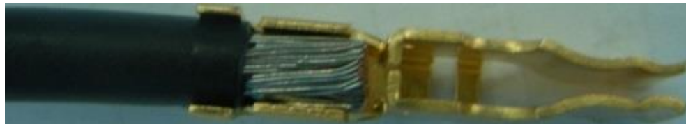
Picture 4. Wire and Terminal before Crimping
