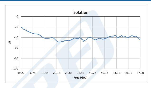
SPST PIN Diode Switch Operating From 50 MHz to 67 GHz Up to +27 dBm and 1.85mm from Pasternack Enterprises has same day shipment for domestic and International orders. Our RF, microwave and millimeter wave products maintain a 99% availability and are part of the broadest selection in the industry.
