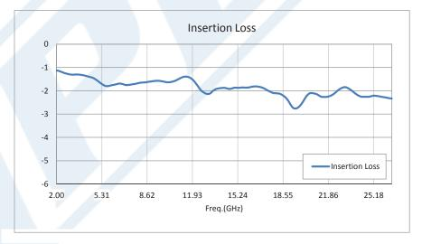
Click the following link (or enter part number in "SEARCH" on website) to obtain additional part information including price, inventory and certifications: SMA SPDT PIN Diode Switch Operating From 2 GHz to 26.5 GHz Up To +30 dBm PE71S2017
