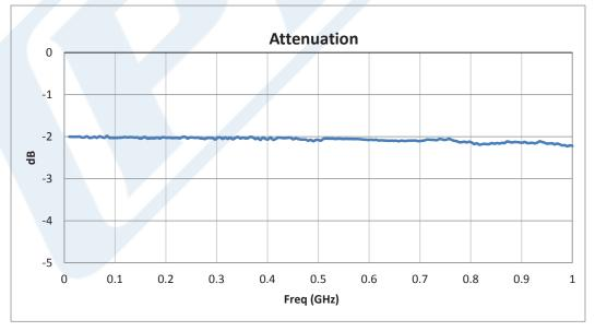
Click the following link (or enter part number in "SEARCH" on website) to obtain additional part information including price, inventory and certifications: 2 dB Fixed Attenuator, 75 Ohm BNC Male to 75 Ohm BNC Female Brass Nickel Body Rated to 1 Watt Up to 1,000 MHz PE7009-2
