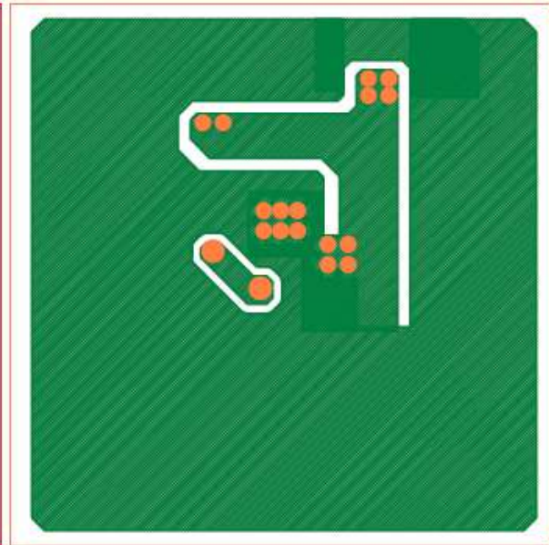
Back Side: GND Side (double sided board)
