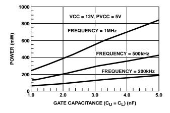
FIGURE 7. POWER DISSIPATION vs FREQUENCY (HIP6601B)
