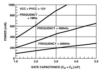
FIGURE 3. POWER DISSIPATION vs LOADING
