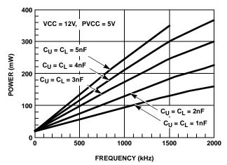
FIGURE 4. POWER DISSIPATION vs FREQUENCY (HIP6603B)
