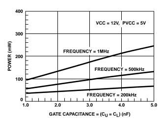
FIGURE 6. VARIABLE LOADING PROFILE (HIP6603B)
