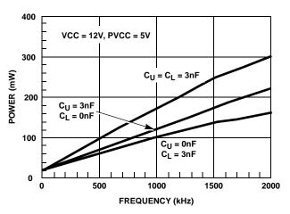
FIGURE 5. 3nF LOADING PROFILE (HIP6603B)
