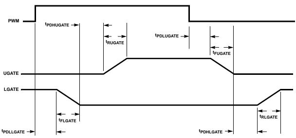
A falling transition on PWM indicates the turn-off of the upper MOSFET and the turn-on of the lower MOSFET. A short propagation delay [tpDLUGATE] is encountered before the upper gate begins to fall [tFUGATE]. Again, the adaptive shoot-through circuitry determines the lower gate delay time, tpDHLGATE. The PHASE voltage is monitored and the lower gate is allowed to rise after PHASE drops below 0.5V. The lower gate then rises [tRLGATE], turning on the lower MOSFET.
