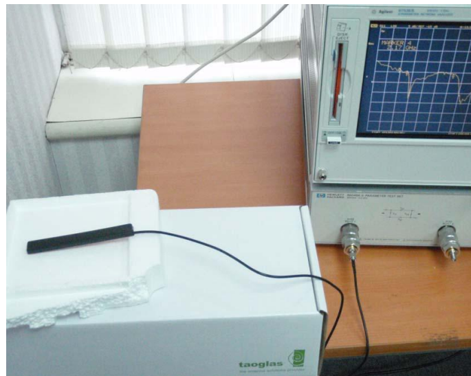
Free space Return Loss measurement setup
