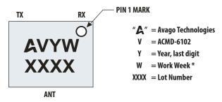
Figure 3. Product Marking and Pin Orientation
