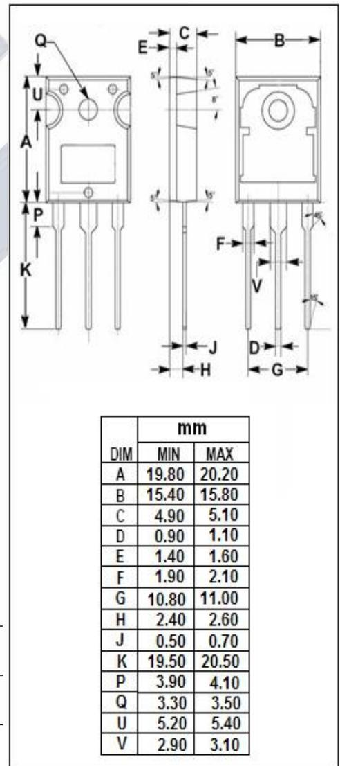
**isc N-Channel MOSFET Transistor**
