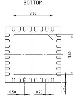
All dimensions given in mm. Tolerances of form and position according to JEDEC MO-220. Positional tolerance of sensor pattern: ±70µm / ±1° (with respect to center of backside pad). G4: radius of chip center (refer to the relevant encoder disc and code description). Maximum molding excess +20µm / -75µm versus surface of glass/reticle.
