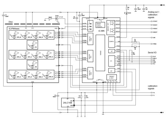
Figure 1: Application example of absolute encoder circuit.
