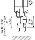
Cable socket M12 with cable (left) and cable plug M12 with cable (right, optional, only on receiver)
