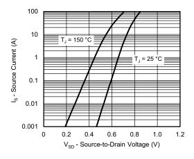
Source-Drain Diode Forward Voltage
