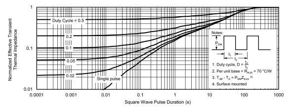
Normalized Thermal Transient Impedance, Junction-to-Ambient
