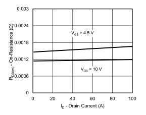
**On-Resistance vs. Drain Current**
