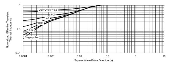
Normalized Thermal Transient Impedance, Junction-to-Case
