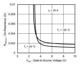
**On-Resistance vs. Gate-to-Source Voltage**
