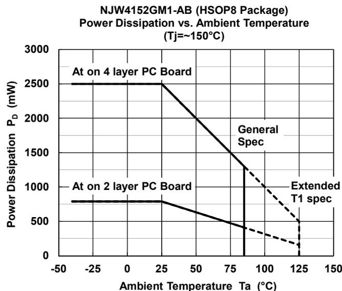
Mounted on glass epoxy board. (76.2×114.3×1.6mm:based on EIA/JDEC standard, 2Layers)
