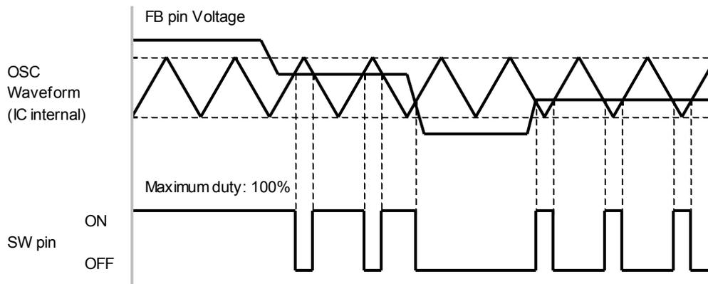
Fig. 1. Timing Chart PWM Comparator and SW pin
