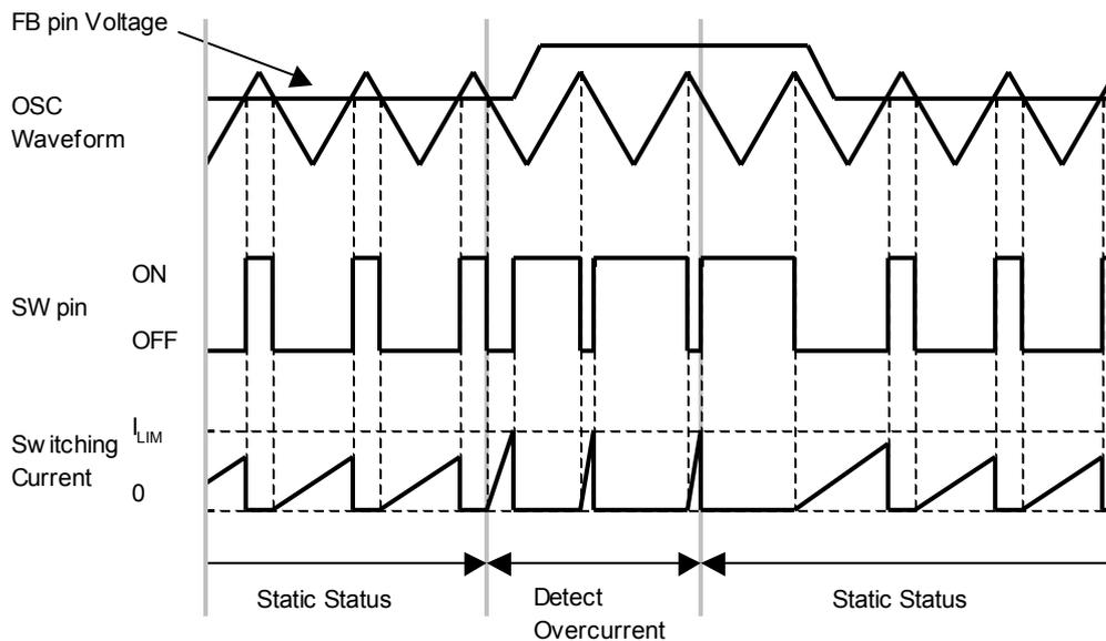
Fig. 3. Timing Chart at Over Current Detection
