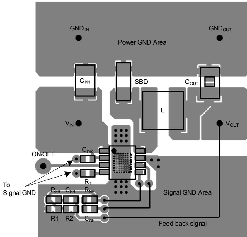
Connect Signal GND line and Power GND line on backside pattern
