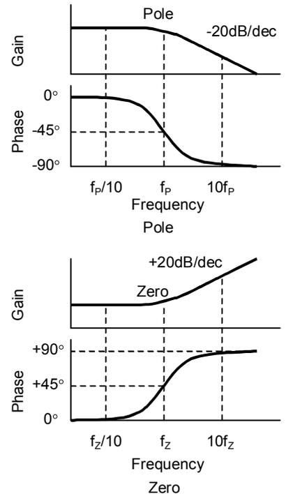
Fig. 10. Characteristics of Pole and Zero
