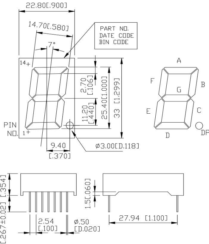
NOTES: All dimensions are in millimeters. Tolerance is  $\pm 0.25$  mm (0.01") unless otherwise noted.
