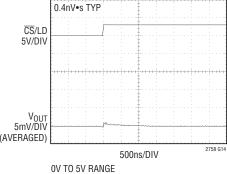
Mid-Scale Glitch  $(V_{DD} = 3V)$
