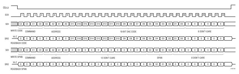
Figure 2. Serial Input and Output Sequences
