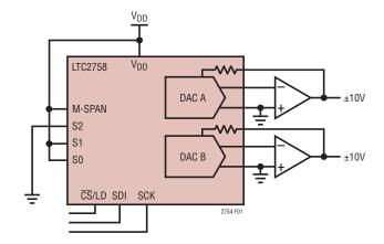
Figure 1. Using M-SPAN to Configure the LTC2758 for Single-Span Operation (±10V Range Shown)
