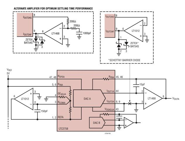
Figure 4. Optional Circuits for Driving  $I_{OUT2}$  from GND with a Force/Sense Amplifier
