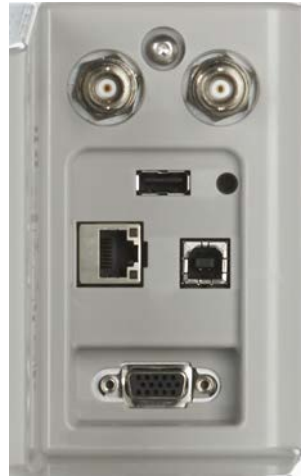
Figure 52. Connectivity section on the back panel.
