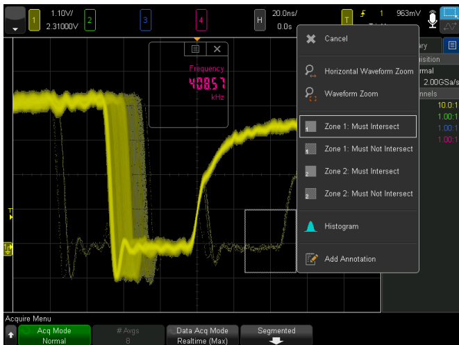
Figure 11. Draw a zone (box) around the anomaly.
