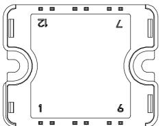
All multiple inputs and outputs must be shorted together 3/4; 5/6; 7/8; 1/2; 9/10
