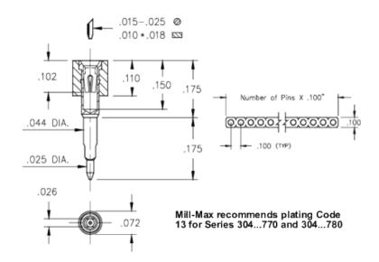
**Description:** Interconnect Socket Solderless Press-Fit Socket Accepts .015"- .025" (0,38 - 0,635
