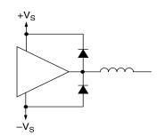
FIGURE 2. PROTECTION, INDUCTIVE LOAD
