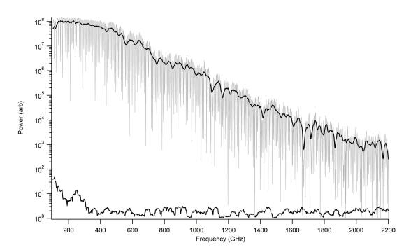
Typical performance of a PB7220-2000 - THz Spectrometer for a scan of laboratory air at 1 ATM. 1 sec time constant.
