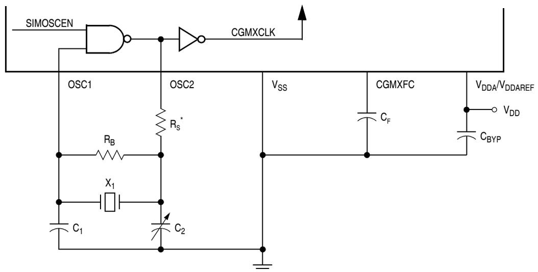
\* $R_S$  can be 0 (shorted) when used with higher-frequency crystals. Refer to manufacturer's data.
