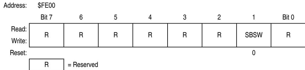
**Figure 13-18. SIM Break Status Register (SBSR)**
