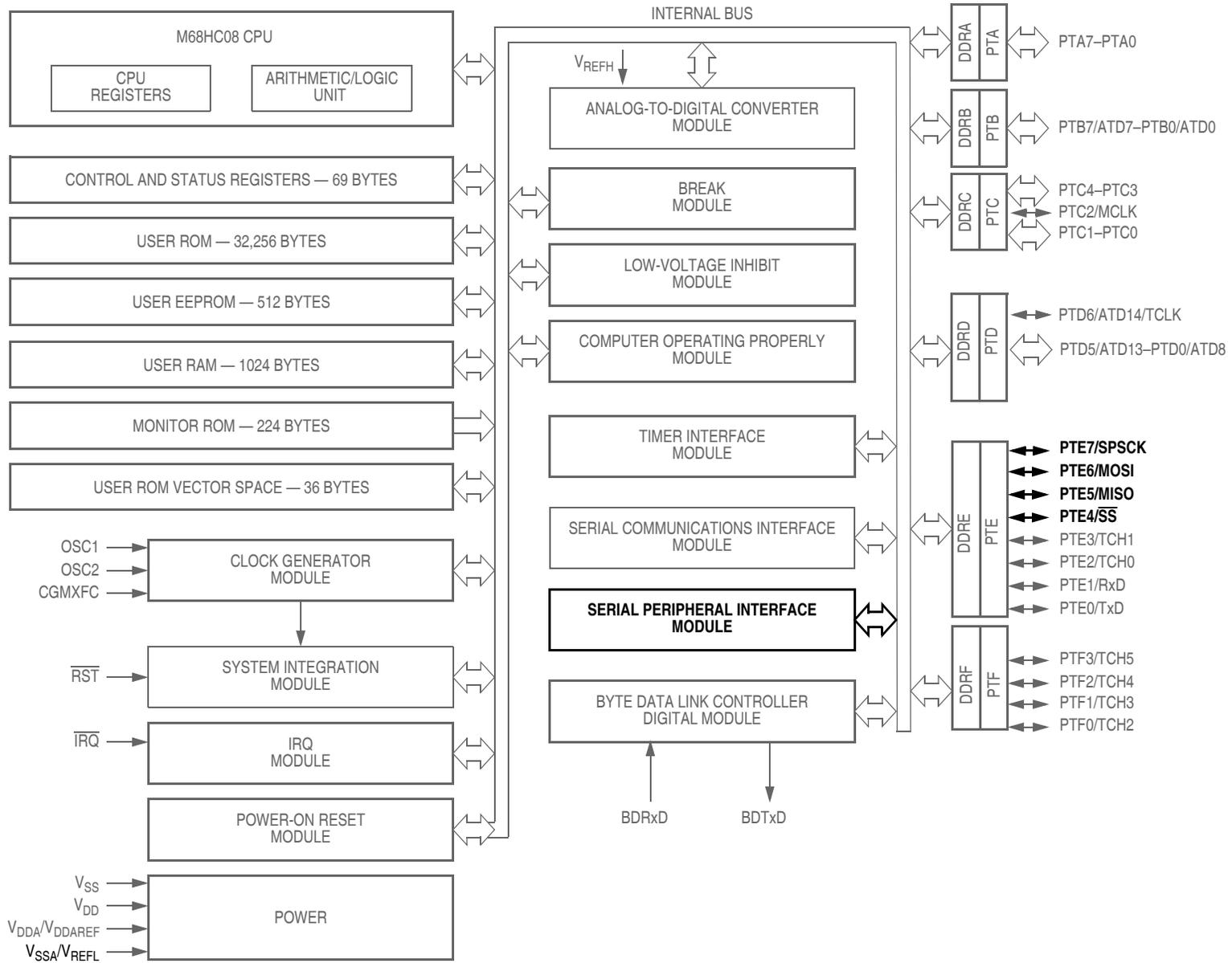
Figure 14-1. Block Diagram Highlighting SPI Block and Pins
