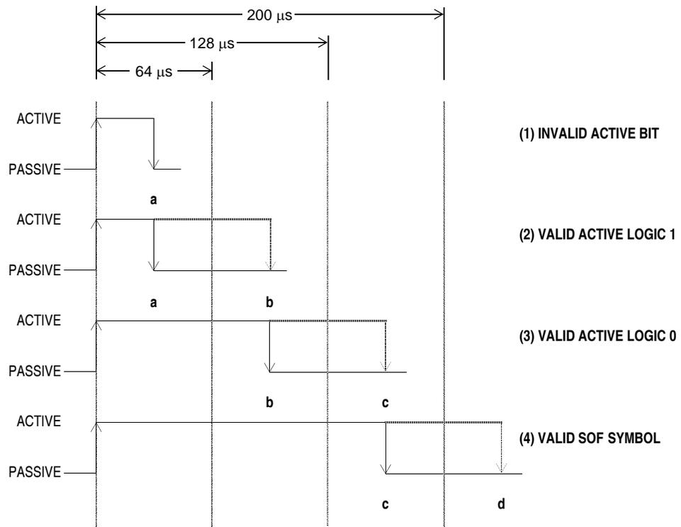
**Figure 4-11. J1850 VPW Received Active Symbol Times**
