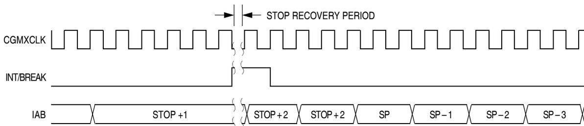
**Figure 13-17. Stop Mode Recovery from Interrupt or Break**
