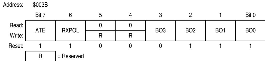
**Figure 4-17. BDLC Analog and Roundtrip Delay Register (BARD)**
