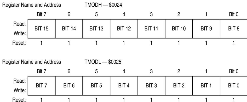
**Figure 15-7. TIM Counter Modulo Registers (TMODH and TMODL)**
