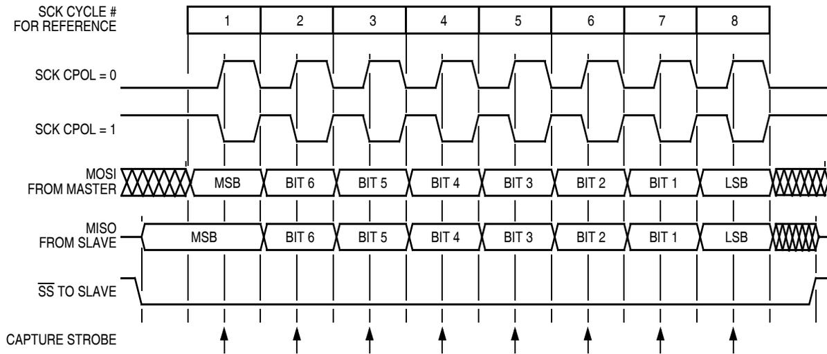
**Figure 14-5. Transmission Format ( $CPHA = 0$ )**
