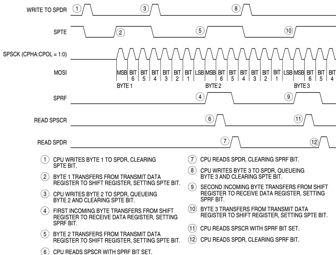
**Figure 14-12. SPRF/SPT E CPU Interrupt Timing**
