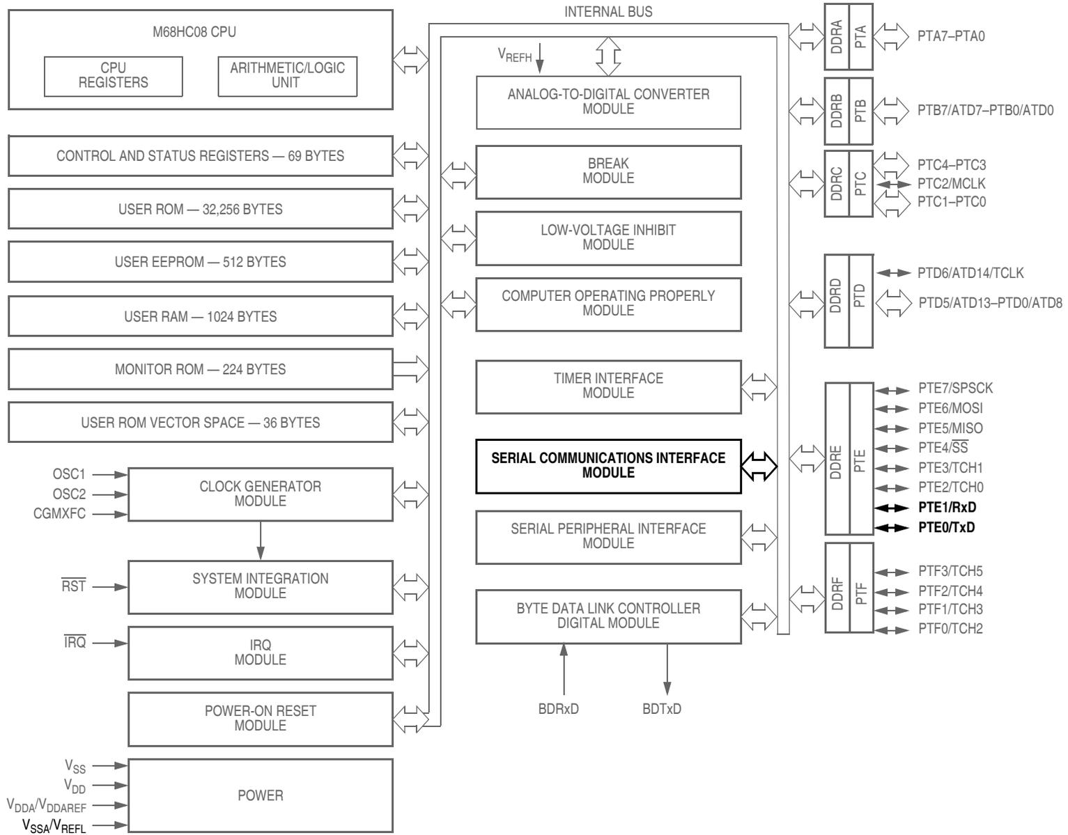
Figure 12-1. Block Diagram Highlighting SCI Block and Pins
