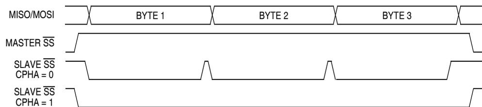
**Figure 14-6.  $CPHA/\overline{SS}$  Timing**
