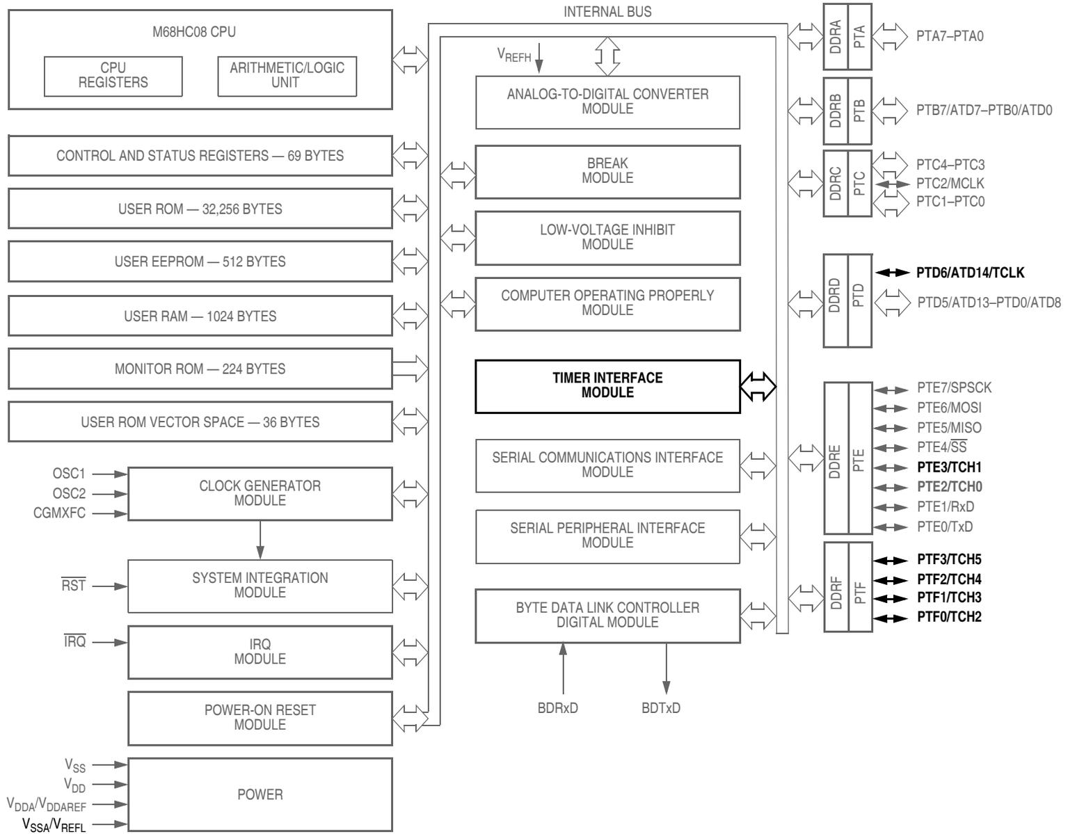
Figure 15-1. Block Diagram Highlighting TIM Block and Pins
