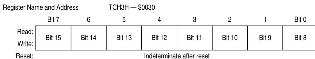
**Figure 15-10. TIM Channel Registers (TCH0H/L–TCH3H/L) (Sheet 1 of 2)**
