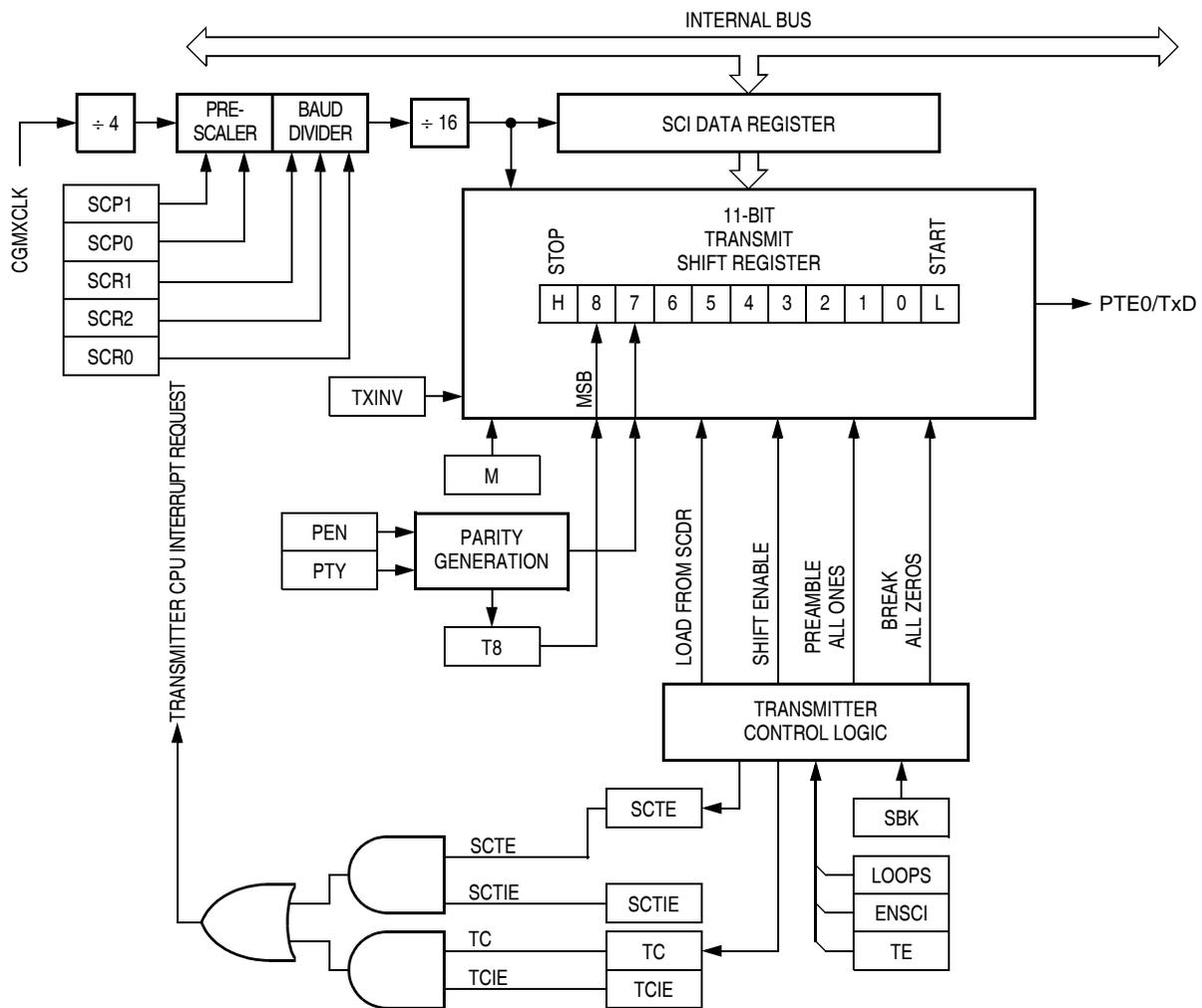
**Figure 12-5. SCI Transmitter**
