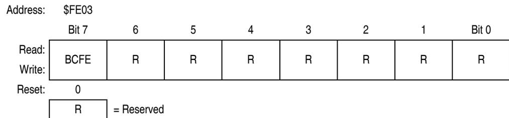
**Figure 13-20. SIM Break Flag Control Register (SBFCR)**
