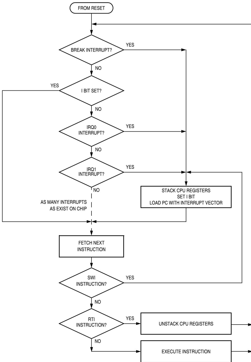
**Figure 13-11. Interrupt Processing**
