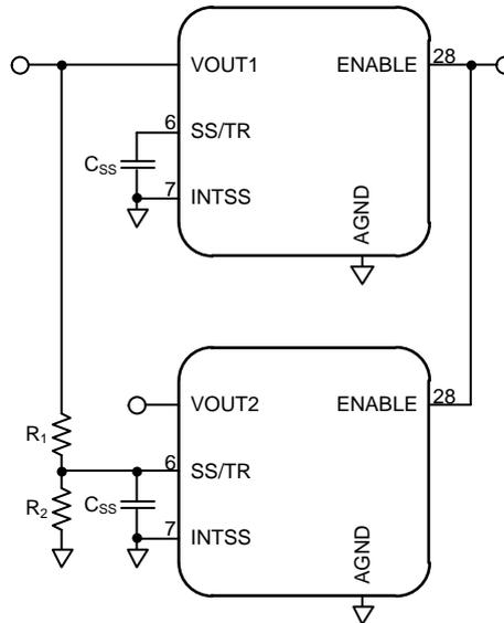
$$R_1 = \frac{V_{OUT2} * 12.6}{0.803} \text{ (k}\Omega\text{)} \quad (7)$$
