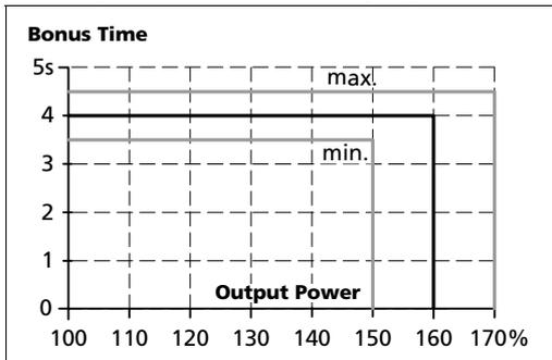
Fig. 6-4 **Dynamic overcurrent capability, typ.**
