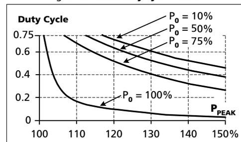
$$\text{DutyCycle} = \frac{T_{\text{peak}}}{T_{\text{peak}} + T_0}$$
