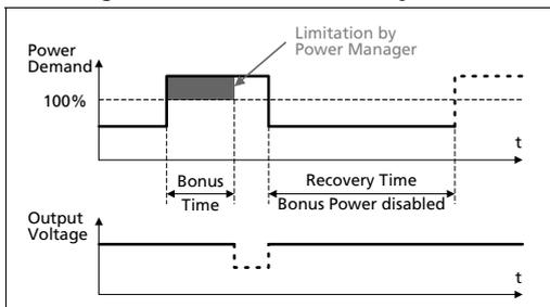
The BonusPower® is available as soon as power comes on and after the end of an output short circuit or output overload.
