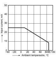
2. Load current vs. ambient temperature char-
