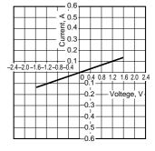
10. Off state leakage current Measured portion: between terminals 4 and 6; Ambient temperature: 25°C 77°F
