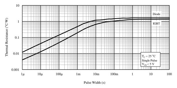
Figure 18. Transient Thermal Resistance
