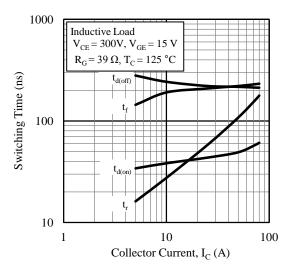
Figure 16. Switching Time vs. Collector Current
