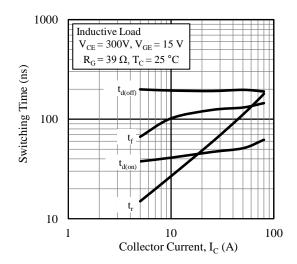
Figure 15. Switching Time vs. Collector Current
