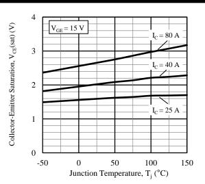
Figure 8. Saturation Voltage vs. Junction Temperature
