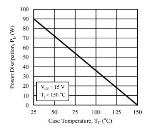
Figure 3. Power Dissipation vs. Case Temperature
