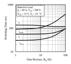
Figure 13. Switching Time vs. Gate Resistor
