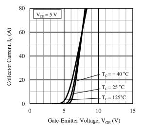
**Figure 7. Transfer Characteristics**
