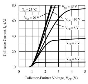
Figure 5. Output Characteristics ( $T_C = 25 \ ^{\circ}C$ )
