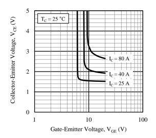
Figure 9. Collector-Emitter Voltage vs. Gate-Emitter Voltage
