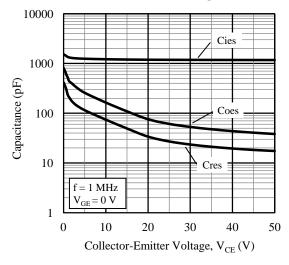
**Figure 11. Capacitance Characteristics**
