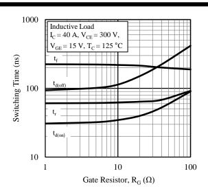
Figure 14. Switching Time vs. Gate Resistor
