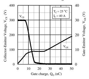
Figure 12. Gate Charge Characteristics
