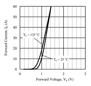
Figure 17. Diode Forward Characteristics
