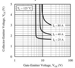
Figure 10. Collector-Emitter Voltage vs. Gate-Emitter Voltage
