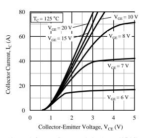
Figure 6. Output Characteristics (T<sub>C</sub> = 125 °C)
