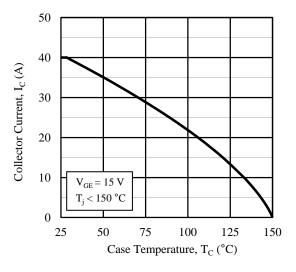
Figure 4. Collector Current vs. Case Temperature
