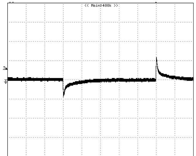
Figure 24: Typical transient response to step load change at 1A/\mu S from 100%~ 50%~100% of I_o , max at 12V_{in} , 0.59V_{out} ( C_{out} = 1\mu F + 47\mu F + 10\mu F ceramic) CH1 : VOUT, 50mV/div, 200uS/div
