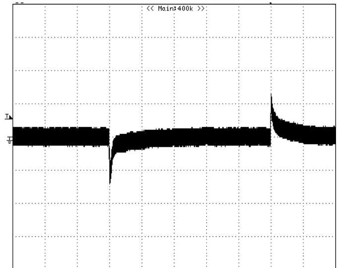
Figure 20: Typical transient response to step load change at 1A/μS from 100%~ 50%~100% of Io, max at 12Vin, 3.3Vout (Cout = 1uF ceramic, 47uF+10μFceramic) CH1 : VOUT, 50mV/div, 200uS/div
