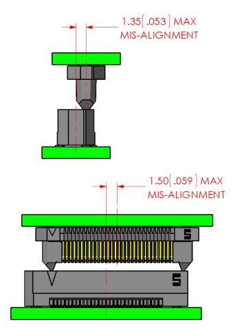
**7.1.2** The parts can be rigidly misaligned by no more than 0,06mm (.002") in the X- and 0,05mm (.002") in the Y-direction to ensure a good mate.
