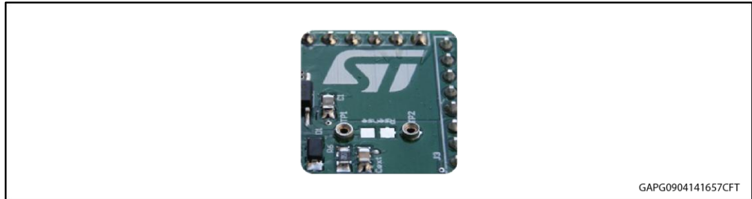
Figure 4: Mounting through-hole sense resistor
