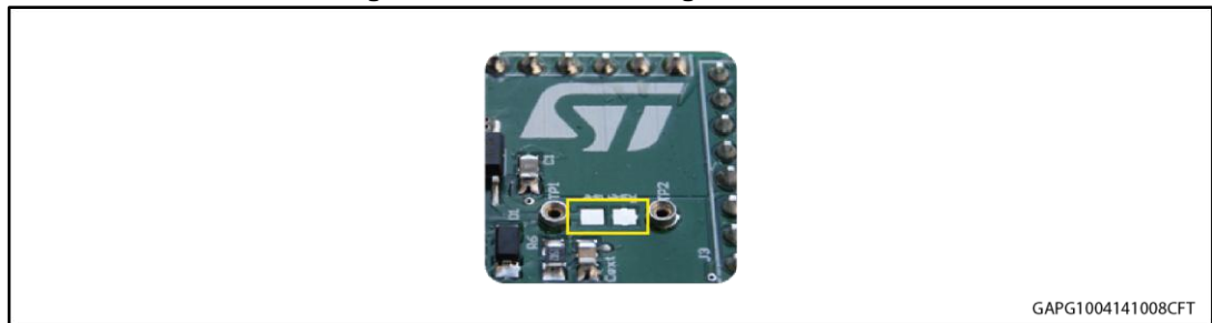
Figure 5: Pads for soldering SMD resistor
