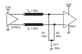
Figure 24: 3.3V LVPECL Output Termination
