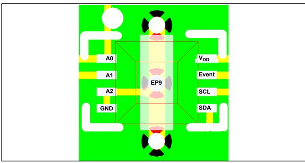
FIGURE 6-1: DFN Package Layout.
