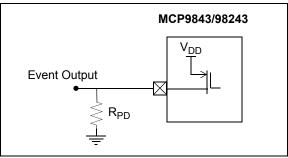
**FIGURE 5-10:** Active-High Event Output Configuration.
