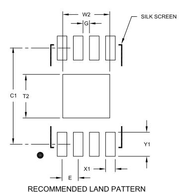
Units MILLIMETERS NOM MAX **Dimension Limits** MIN Contact Pitch Ε 0.50 BSC Optional Center Pad Width W2 1.46 Optional Center Pad Length 1.36 T2 Contact Pad Spacing C1 3.00 Contact Pad Width (X8) Χ1 0.30 Contact Pad Length (X8) Υ1 0.75 Distance Between Pads G 0.20
