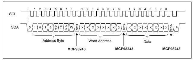
FIGURE 5-13: Timing Diagram for Byte Write (See Section 4.0 "Serial Communication").
