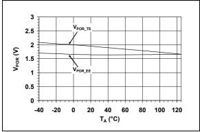
**FIGURE 2-6:** Power-on Reset Threshold Voltage vs. Temperature.
