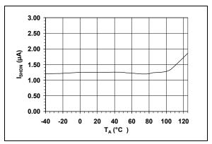
**FIGURE 2-14:** Shutdown Current vs. Temperature.
