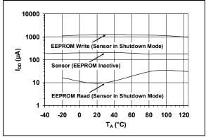
FIGURE 2-4: Supply Current vs. Temperature.
