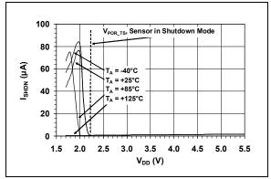
FIGURE 2-15: Shutdown Current vs. V<sub>DD</sub>.
