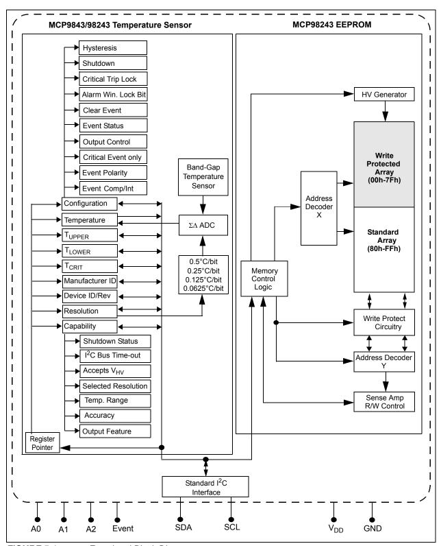
FIGURE 5-1: Functional Block Diagram.
