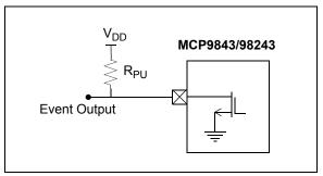
**FIGURE 5-11:** Active-Low Event Output Configuration.
