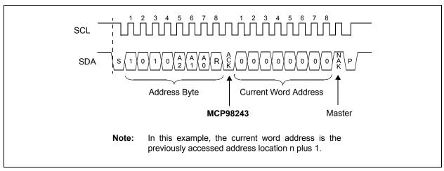
FIGURE 5-18: Reading Current Word Address (See Section 4.0 "Serial Communication").
