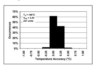
**FIGURE 2-2:** Temperature Accuracy Histogram,  $T_A = +95$ °C.
