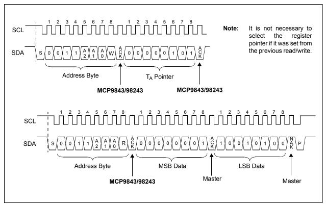
**FIGURE 5-7:** Timing Diagram for Reading  $+25.25^{\circ}$ C Temperature from the  $T_A$  Register (See **Section 4.0 "Serial Communication"**).
