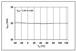
**FIGURE 2-5:** Serial Bus Time-Out vs. Temperature.
