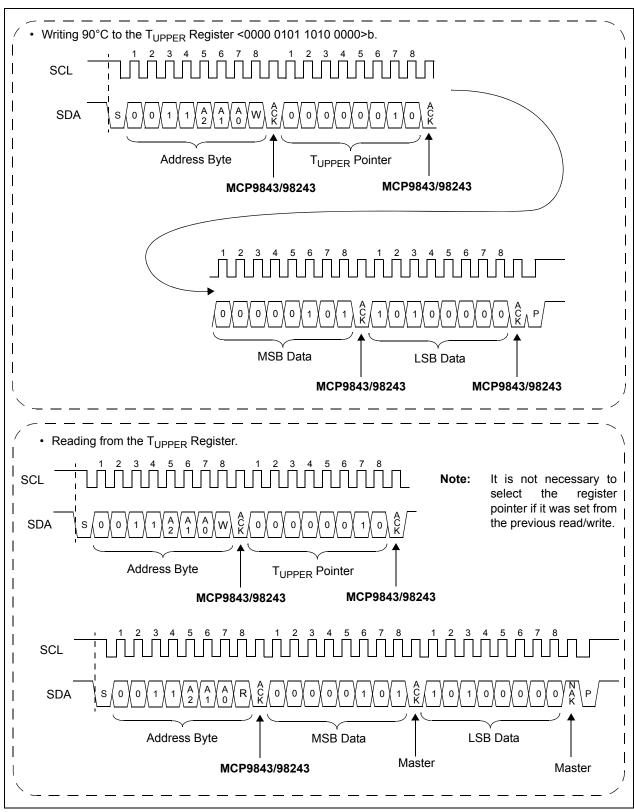
**FIGURE 5-5:** Timing Diagram for Writing and Reading from the T<sub>UPPER</sub> Register (See **Section 4.0** "Serial Communication").
