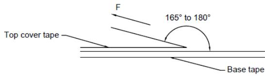
The force for tearing off cover tape is 15 to 60 grams in the arrow direction under the following conditions.
