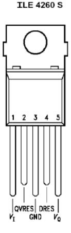
Pin Definitions and Functions (ILE 4260 and ILE 4260 S)
