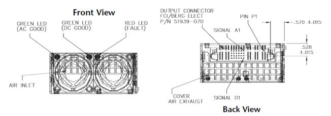
Input: 90Vac to 264Vac; Output: -54Vdc @ 1200W
