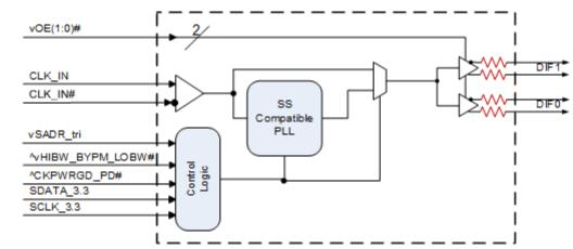
Note: Resistors default to internal on xx42/xx52 devices. P2 devices have programmable default impedances on an output-by-output basis.
