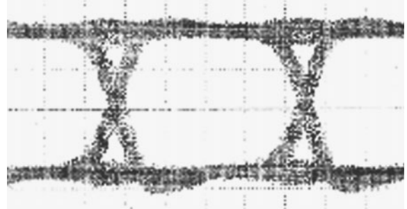
(Figure 2) Tracing of the same signal after equalization. Receiver output measured at pins 2 and 3.
