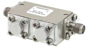
Dual Junction Isolator With 40 dB Isolation From 11 GHz to 18 GHz, 5 Watts And SMA Female
